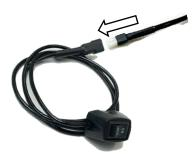
**Step 22:** Locate the black wires for the disable switch and feed them to your desired mount location. Prepare the surface by cleaning with a 50/50 mix of isopropyl alcohol and water or equivalent. Once the surface is dry, peel the backing from the double-sided tape and stick the disable switch on the lower dash panel. Plug the disable switch connector into the black wire harness and tuck the extra wire behind the lower dash panel.
