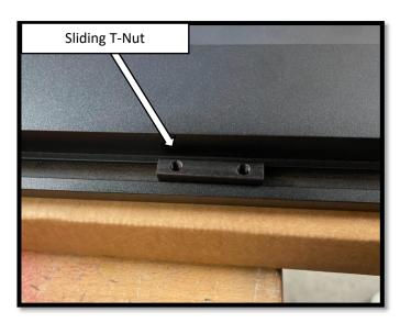
**Step 8**: Install the passenger side running board. With assistance, begin by positioning the board on the front and rear motor assembly bases. Align the sliding T-Nut on the running board with the slots on the front and rear motor base. Once the T-Nuts are aligned, rotate the running board so that the T-Nuts set in the slots on the base of the arms.
