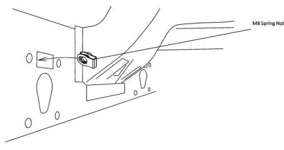
**Step 4**: Install the rear Passenger side motor using (2) hex bolts, (2) M8 Flat Washers, (2) M8 Lock Washers and (2) M8 Spring into the upper mounting holes of the rocker panel to fasten the motor to the truck. The hardware should be hand tightened only until snug. This will allow the motor assembly to move and align easier when installing the running board.
