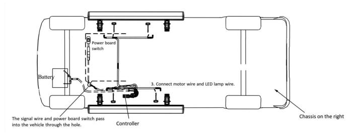
**Step 13**: Route the motor and LED wire harness from the controller to the Driver side frame rail of the vehicle. When routing the harness keep clear from any moving parts and avoid direct contact with the exhaust system.
