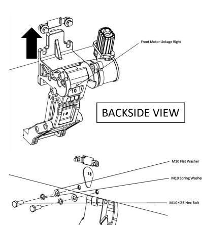
**Step 5**: Install the Front Passenger side motor using (2) hex bolts, (2) M8 Flat Washers, (2) M8 Lock Washers into the front mounting holes of the pinch weld to fasten the motor to the truck. The hardware should be hand tightened only until snug. This will allow the motor assembly to move and align easier when installing the running board.
