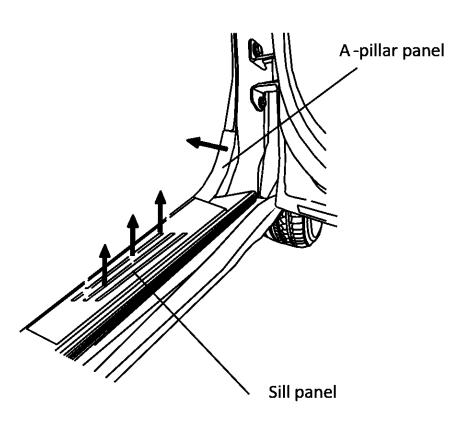
Step 14: On the Passenger side, remove the front kick panel, front door sill trim panel, and b-pillar trim panel. Pull the front passenger carpet back and cut a 7/16" hole on the rubber gromet as shown. Feed the door trigger signal wires (white and brown) and the disable switch wires (two black wires) into the cab. Seal around the wires using RTV silicone adhesive to prevent water intrusion.
